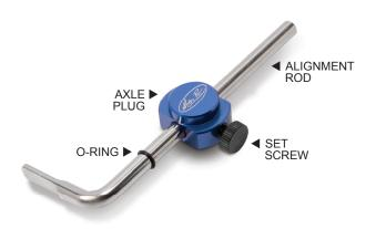
**1.** Loosen knurled set screw to allow the alignment indicator rod to move freely in axle plug.
